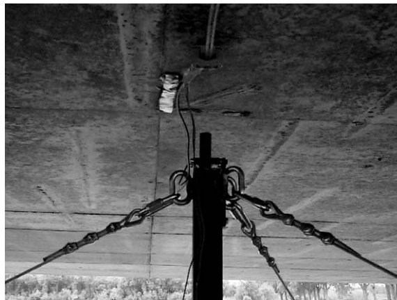
Fig. 5. Installation of LVDT and strain gauges.
